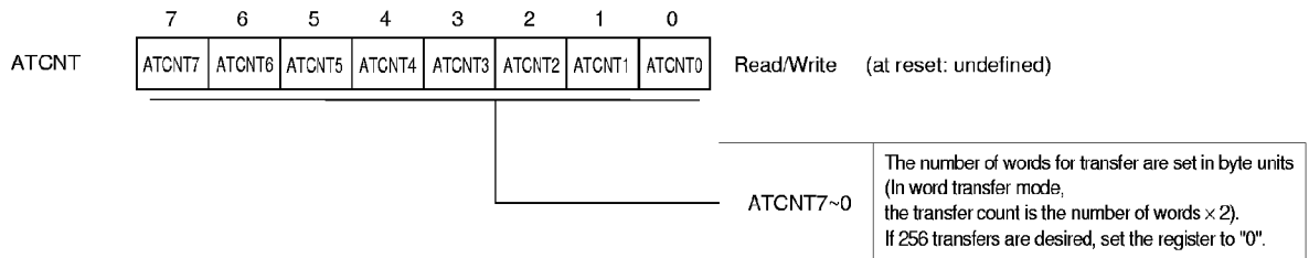
Figure 8-3-2 Transfer Word Counter (ATCNT: X'03FA1', R/W)
